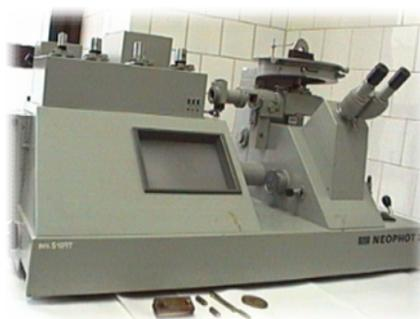
Fig. 3 – Optical metallographic microscope Neophot® 21 – bird's-eye view.
