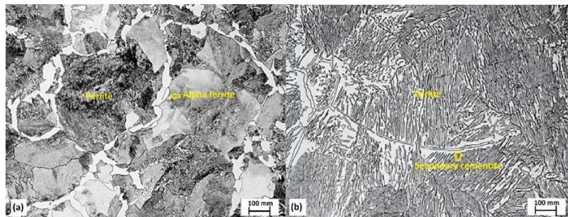
Fig. 1 – Typical microstructures of plain carbon steels: (a) hypoeutectoid; (b) hypereutectoid (Mackenzie, 2025).
