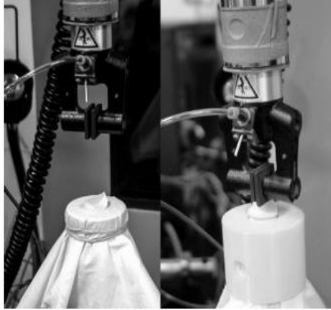
Fig. 4 – Adhesion testing assembly (source: Rivera et al. , 2017).
