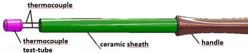
Fig. 3 – Ag cylindrical specimen of standardized dimensions with chromel-alumel type thermocouple embedded in the center having the following characteristics:  $\varnothing = 13$  [mm];  $h = 28$  [mm];  $S = 1408$  [mm<sup>2</sup>];  $m = 39.9$  [g];  $\rho_{Ag} = 10.5$  g/cm<sup>3</sup>;  $\lambda_{Ag} = 418.5$  W/m·K.
