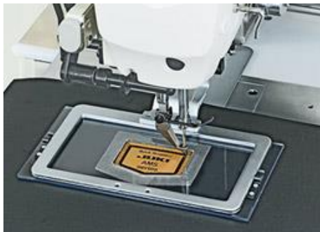
Fig. 2 – Close-up of the AMS machine applying a later by using a pressing plate (Linz et al. , 2005).
