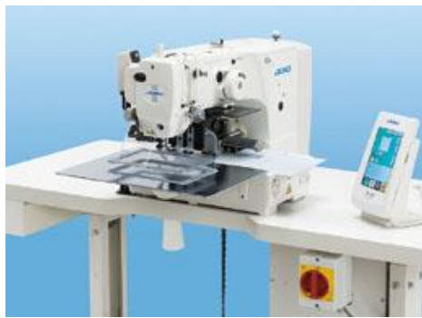
Fig. 1 – Juki AMS CNC sewing machine (Linz et al. , 2005).
