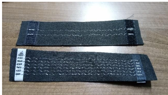
Fig. 5 – Elastic bands with Bekinox circuits and velcro: 2 lines (up) and 6 lines (down).
