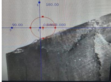
Fig. 11 – Image obtained on Zoller equipment for a drill cutting edge, non uniform wear: infrared light method; – magnification 12 x.
