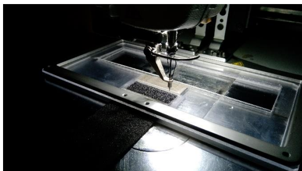
Fig. 6 – AMS machine ready to sew a velcro strip using a custom made holding plate.
