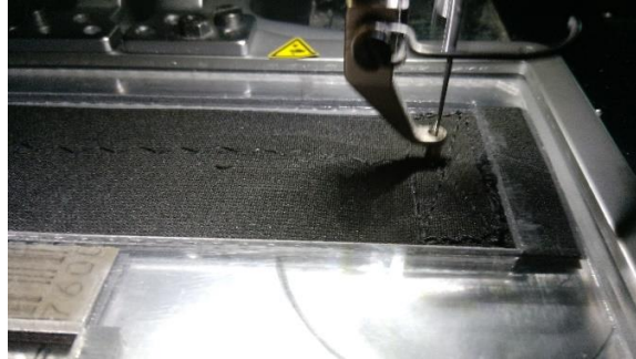
Fig. 7 – AMS machine embroidering on an elastic band.
