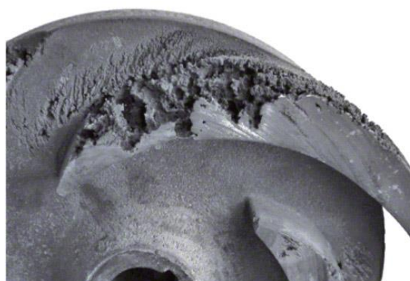
Fig. 6 – Defect due to pitting corrosion.
