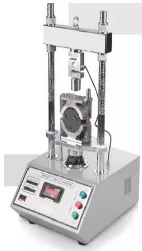
Fig. 3 – Photograph of the Marshal Stability tester ( https://www.multilab.ro/asfalt/aparat_Marshall_50KN.html ).
