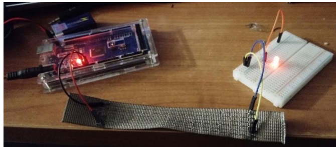
Fig. 8 – Ribbon with Bekinox thread providing power to an LED.
