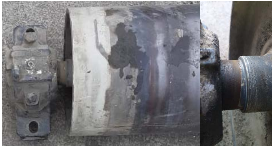
Fig. 6 – Return drum with bearing – left side. Detail of axle neck journal - right side.
