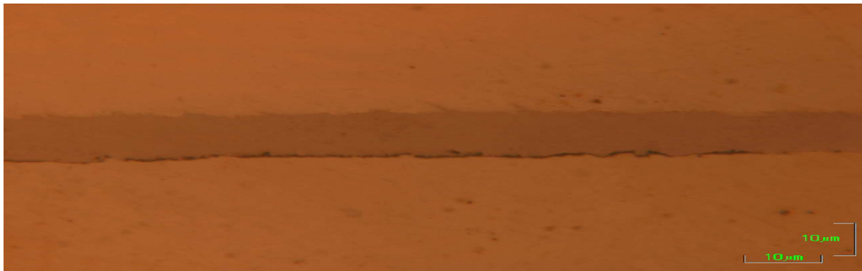
Fig. 10 Cross section of the Al coating on a stainless steel 316, treatment time 45 minutes at 610°C, with HCl activator
