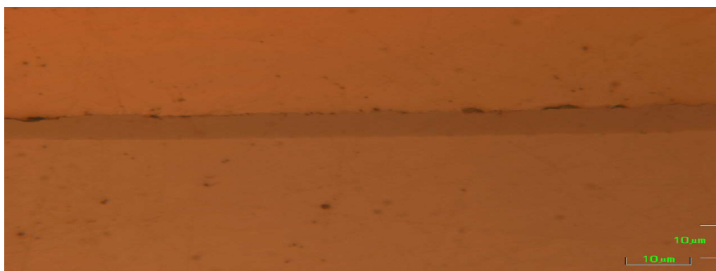
Fig. 9 Cross section of the Al coating on a stainless steel 316, treatment time 30 minutes at 610°C, with HCl activator
