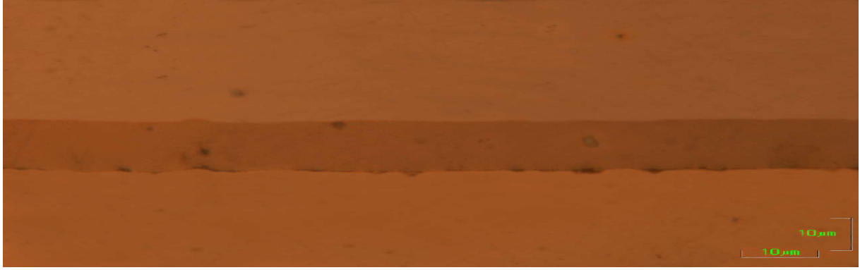
Fig. 4 Cross section of the Al coating on a stainless steel 316, treatment time 120 minutes at 600°C, with HCl activator
