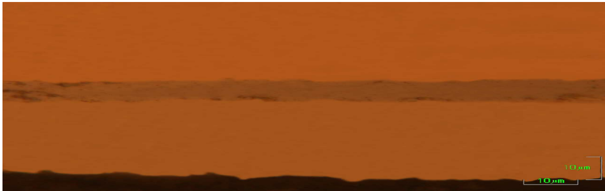
Fig. 2 Cross section of the Al coating on a stainless steel 316, treatment time 30 minutes at 600^\circ\text{C} , with HCl activator
