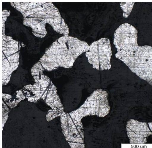
Fig. 7 – Metallographic microscope image of a porous metal structure obtained by sintering the NaCl particles in water vapor for 10 minutes.
