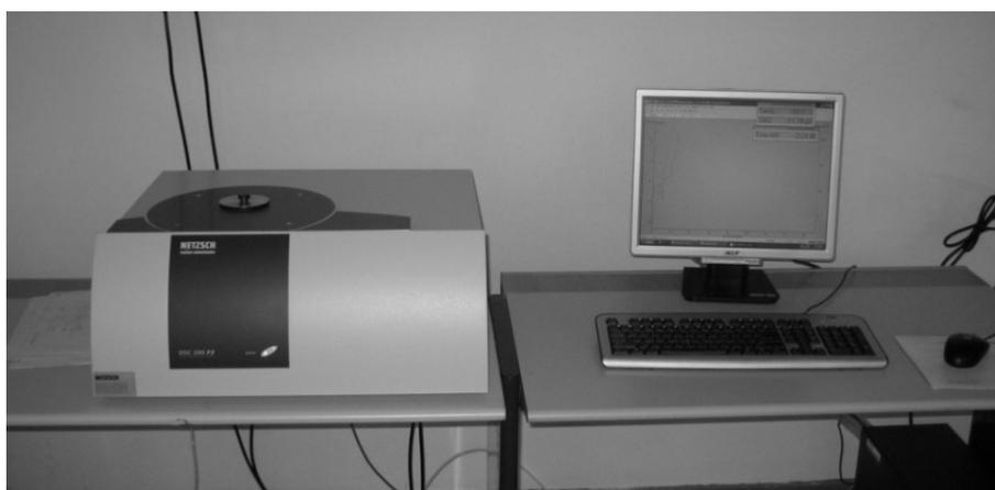
Fig. 1 – Calorimeter DSC F3 Maia.
