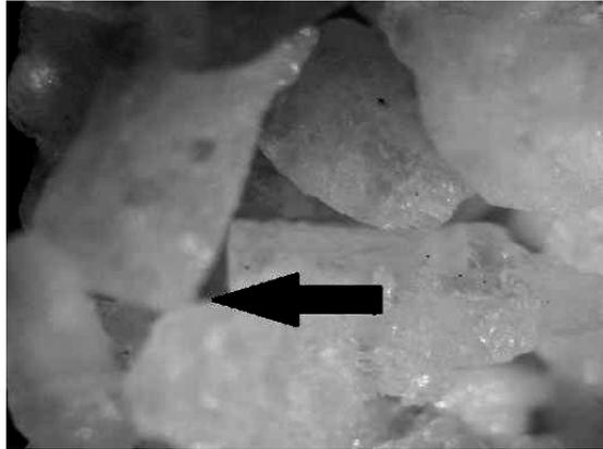
Fig. 3 – Optical microscopy image obtained by sintering salt in air (particles of 1.2–1.6 mm).
