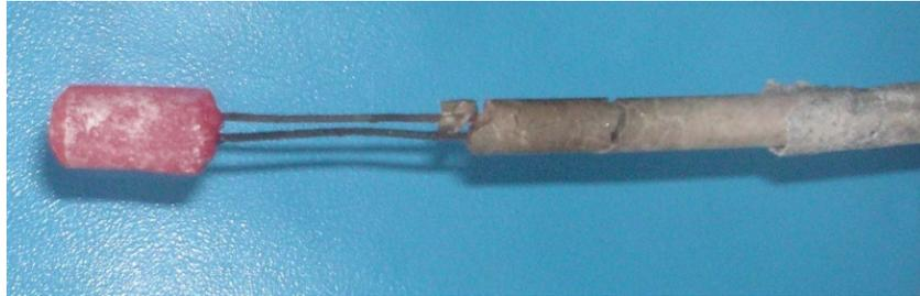
Fig. - 2. Silver samples with the following sizes and features:  $\varnothing = 12,5$  [mm],  $h = 25$  [mm],  $S = 1408$  [mm<sup>2</sup>],  $m = 39.9$  [g],  $\rho_{Ag} = 10.5$  g/cm<sup>3</sup>,  $\lambda_{Ag} = 418.5$  W/m·
