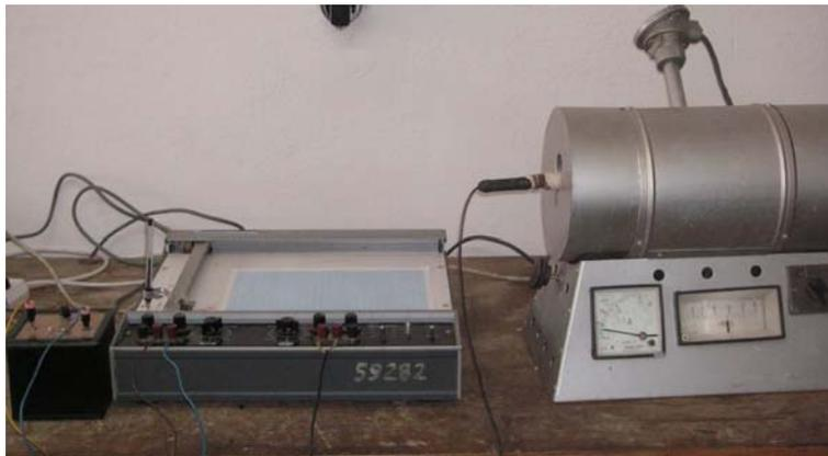
Fig. 1 - Installation for cooling characteristics determination.
